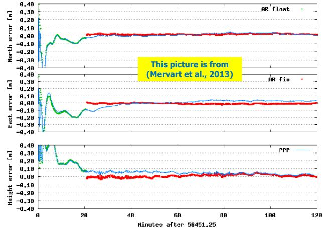
The main weakness of PPP is the large convergence time, which depend on satellites geometry, quality of data (code noise, cycle-slips...). There is a sudden improvement when fixing carrier ambiguities, but still several tens of minutes are needed to achieve centimeter level of accuracy.
