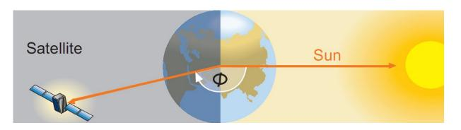
High-accuracy GNSS positioning degrades during the GNSS satellites' eclipse seasons.
