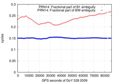
These carrier hardware biases are slow varying parameters and can be broadcast to the user, together with the other differential corrections (orbits, clocks, ionosphere...) from a reference station network.
