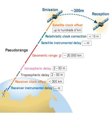
The PPP technique allows centimetrelevel of accuracy to be achieved for static positioning and decimetre level, or better, for kinematic navigation. This high accuracy requires an accurate **modelling "up to the centimetre level or better"**, where all previous model terms must be taken into account (except ionosphere and TGD [\*]), **plus some additional terms given next:**
