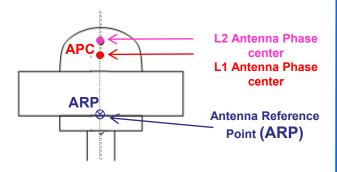
GNSS measurements are referred to the APC. This is not necessarily the geometric center of the antenna, and it depends on the signal frequency and the incoming radio signal direction.
