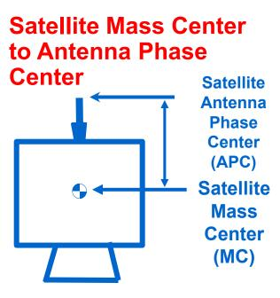
Broadcast orbits are referred to the antenna phase center, but IGS precise orbits are referred to the satellite mass center.
