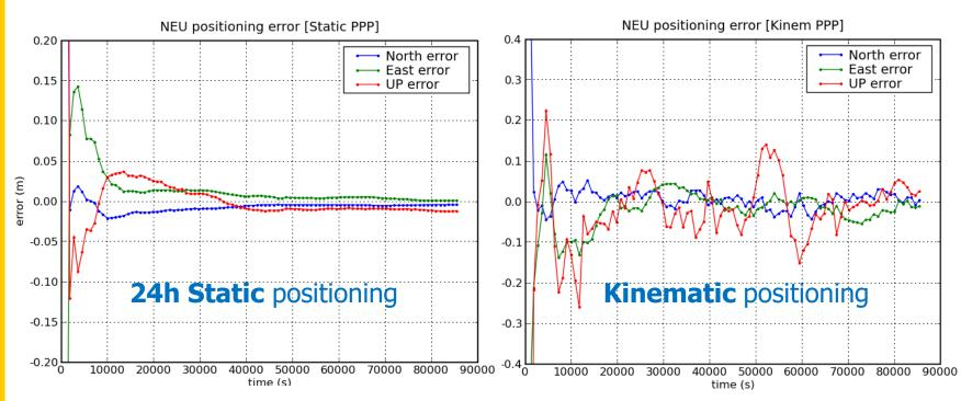
This high accuracy requires the use of code and carrier measurements and an accurate measurement modelling up to centimetre level or better.
