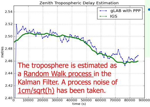
A residual tropospheric delay is estimated (as wet ZTD delay) in the Kalman filter, together with the coordinates, clock and carrier phase ambiguities.
