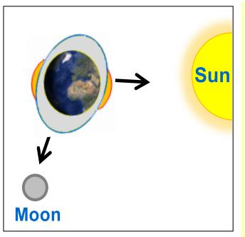
**Solid Tides** concern the movement of Earth's crust (and thus the variation in the receiver's location coordinates) due to gravitational attractive forces produced by external bodies, mainly the Sun and Moon. Solid tides produce vertical and horizontal displacements that can be expressed by the spherical harmonics expansion (m, n), characterised by the Love and Shida numbers  $h_{mn}$  and  $l_{mn}$ .
