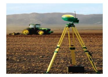
The key feature of RTK is the ability to fix the carrier ambiguities On-The-Flight (OTF), i.e. while on the move. Major receivers manufacturers offer RTK solution packages consisting on a pair or receivers, a radio link, and software. The performance of RTK is measured by (i) initialization time, and (ii) reliability (or, correctness) of the ambiguity fixing. There is an obvious tradeoff between getting the answer quickly and getting it right.
