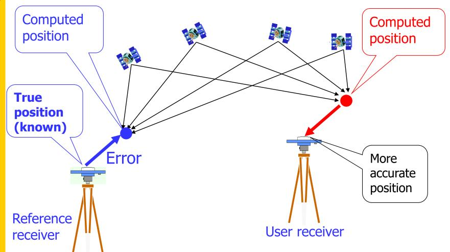
If the coordinates of the reference receiver are known, thence the reference receiver can estimate its positioning error, which can be transmitted to the user. Then, the user can apply these corrections to improve the positioning Note: Actually the corrections are computed in range domain (i.e. for each satellite) instead of in the position domain.
