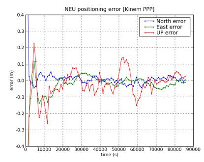
For an observation span relatively long, e.g. one hour, the floated ambiguities (in PPP) would typically be very close to integers, and the change in the position solution from the float to the fixed solution should not be large.
