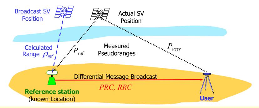
The reference station, with known coordinates , computes range corrections for each satellite in view. These <u>corrections are broadcasted</u> to the user. The user applies these corrections to compute its "absolute position".
