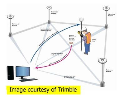
After initialization, the survey proceeds in exactly the same manner as an RTK survey. No receiver upgrade is needed (regarding to RTK).
