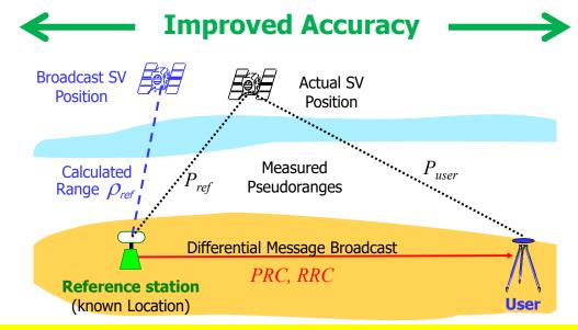
Errors are similar for users separated tens, even hundred of km, and are removed/mitigated in differential mode, improving positioning.
