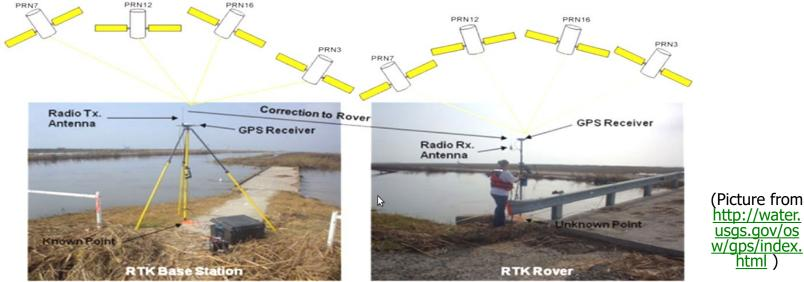
It involves a reference receiver transmitting its raw measurements to a rover receiver via some sort of communication link (e.g. VHF or UHF radio, cellular phone). The data processing at the rover receiver includes ambiguity resolution of the differential carrier data and coordinate estimation of the rover position.
