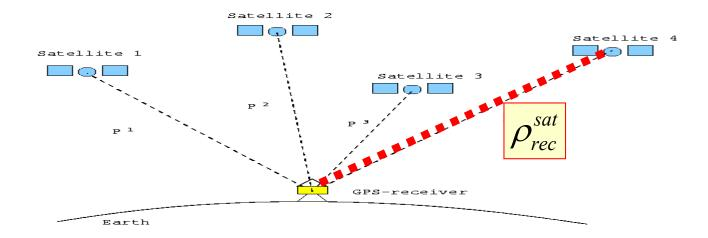
Euclidean distance between satellite coordinates at emission time and receiver coordinates at reception time.
