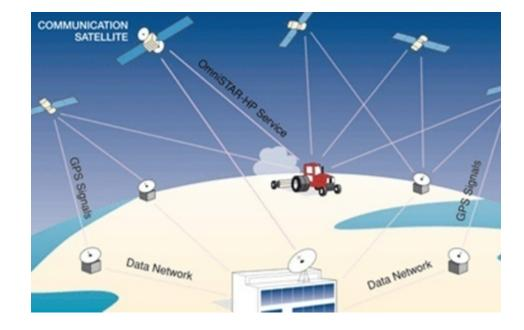
**OmniSTAR HP (10cm)** service is the **most accurate solution** available in the OmniSTAR portfolio of correction solutions. It is a L1/L2 solution requiring a <u>dual frequency</u> receiver.
