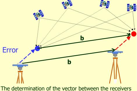
The determination of the vector between the receivers APCs (i.e. the baseline "b') is more accurate than the single receiver solution, because common errors cancel
