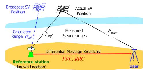
Errors are similar for users separated tens, even hundred of km, and are removed/mitigated in differential mode, improving positioning.
