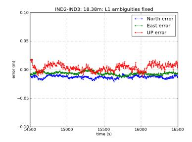
Errors are similar for users separated tens, even hundred of kilometres, and these errors are removed/mitigated in differential mode, improving positioning.
