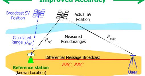
Errors are similar for users separated tens, even hundred of km, and are removed/mitigated in differential mode, improving positioning.
