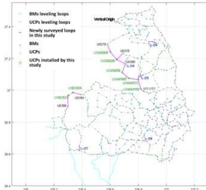
Figure 6. A pilot UCPs-based network to be adjusted.
