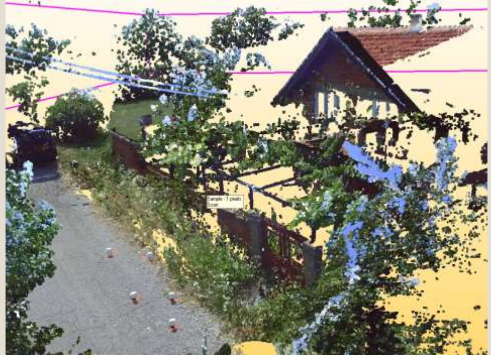
Fig. 10 The second station of the scanner – for the inaccessible rear part of object “A”
