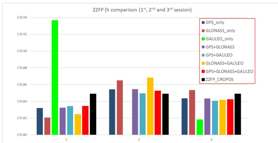
Figure 8. Ellipsoidal heights of station ZZFP obtained from different data combination in 1<sup>st</sup>, 2<sup>nd</sup> and 3<sup>rd</sup> session.
