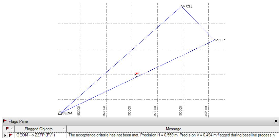
Figure 4. Subnetwork with baselines between stations GEOM, MRGJ and ZZFP processed with Galileo-only satellites observations during the 2<sup>nd</sup> session; a float solution was obtained for the baseline GEOM → ZZFP having not met the Horizontal and Vertical precision acceptance criteria.
