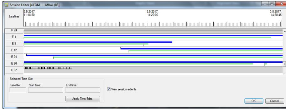
Figure 6. Session editor for the baseline GEOM → ZZFP (2<sup>nd</sup> session); continuous visibility of 4-6 satellites has allowed the determination of a fixed solution.
