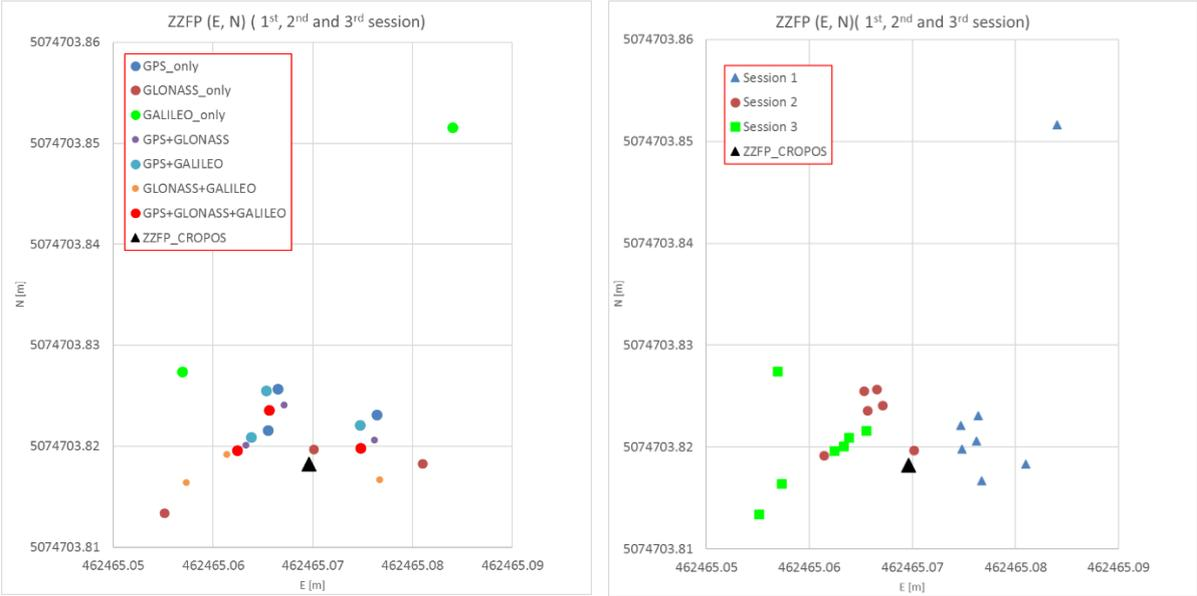
Figure 7. (left): Coordinates of station ZZFP obtained from different data combinations in 3 different sessions; (right): Coordinates of station ZZFP obtained from different data combinations, individually presented for each session (right).
