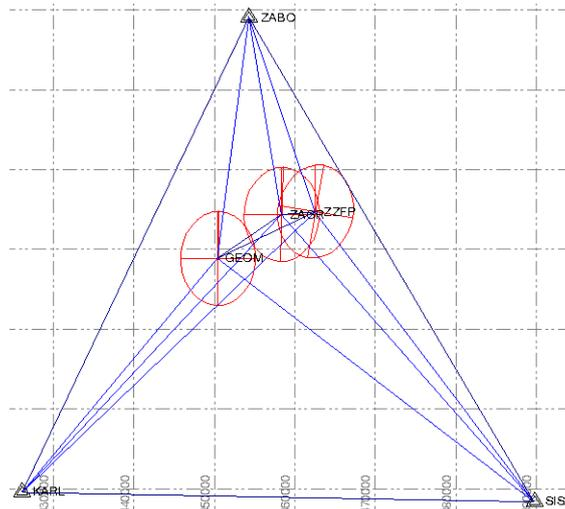
Figure 2. Network with baselines processed with GPS + GLONASS combination after a fully constrained adjustment; the adjustment was performed with uncorrelated vectors.
