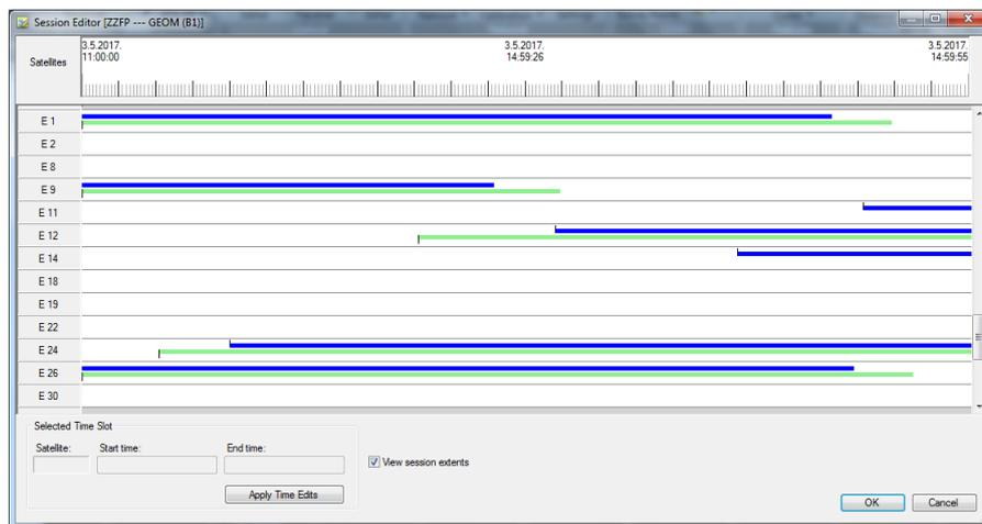
Figure 5. Session editor for the baseline ZZFP → GEOM (2<sup>nd</sup> session); a gap in the visibility of satellites E9 and E12 has most likely prevented a fixed solution.
