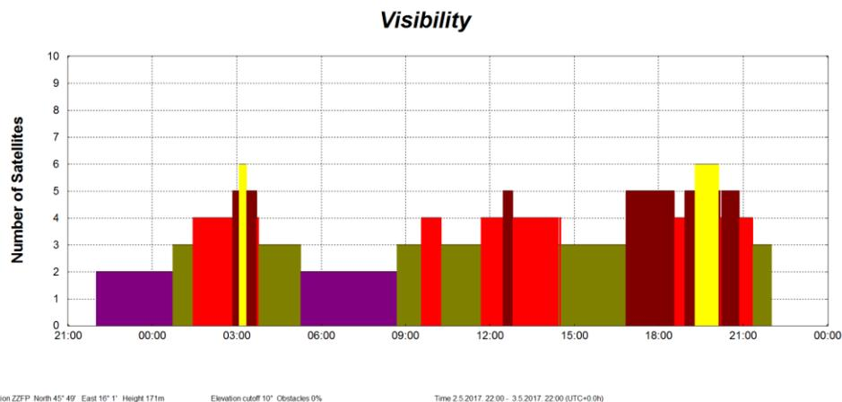
Figure 3. Galileo satellites visibility at the station ZZFP, for May 3<sup>rd</sup> 2017 in period 0-24 CET (22 – 22 UTC).
