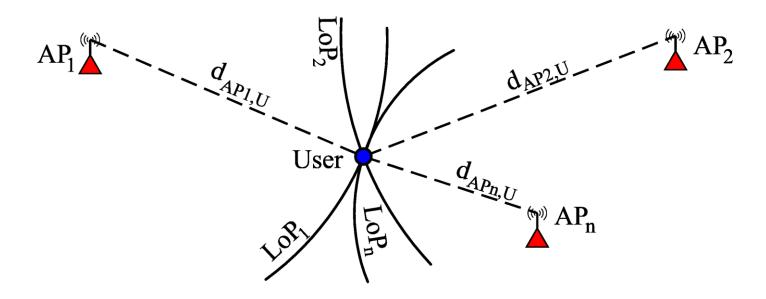
Intersection of at least 3 spherical surfaces given the centres and radii of those spheres
