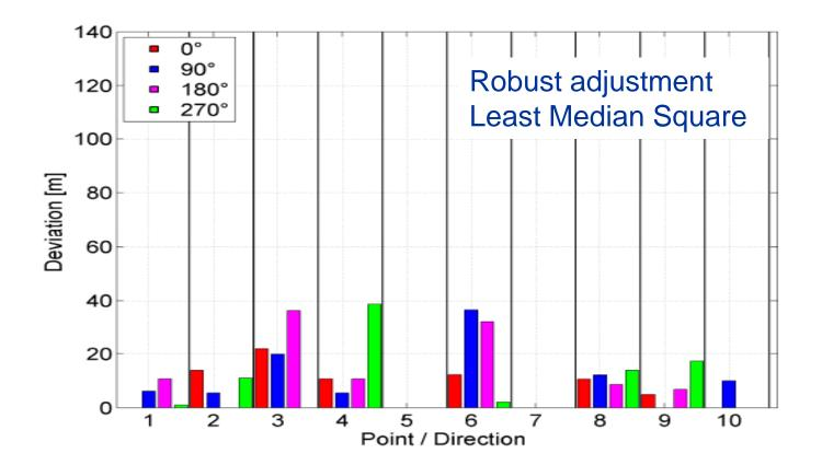
With differential corrections using reference station measurements and consideration of user orientation
