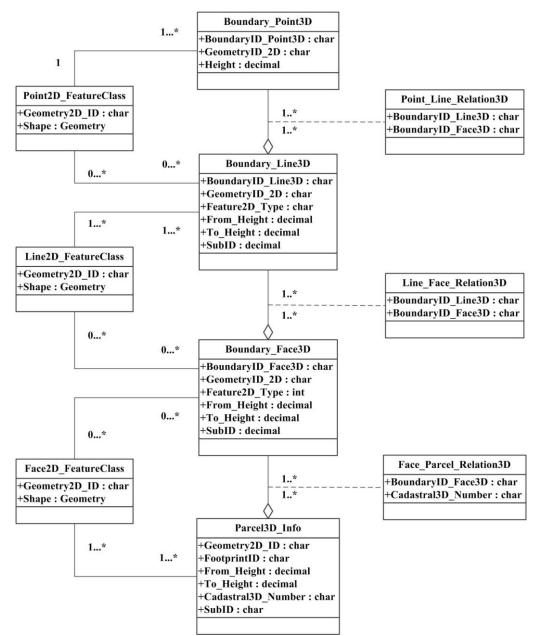
Figure 13: The main physical structure of our 3D cadastral database.
