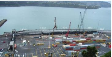
tracking of these points. The application reported the displacement and set off alarms where thresholds were exceeded. The piling operation caused the toe of the embankment under the wharf to fail with a resultant shift of the wharf and building structure.
