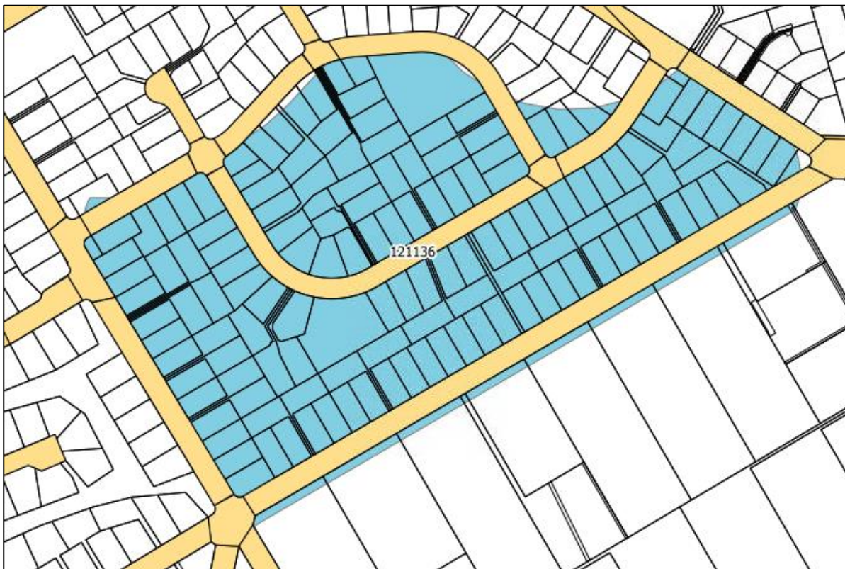
Figure 1: The blue color represents the extent of the parcel block. All cadastral data within and going down the roads that bound the parcel block are brought into the adjustment.
