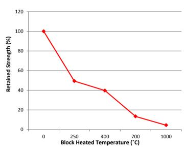
Fig. 6b: Retained Strength vs Block Heated Temperature
