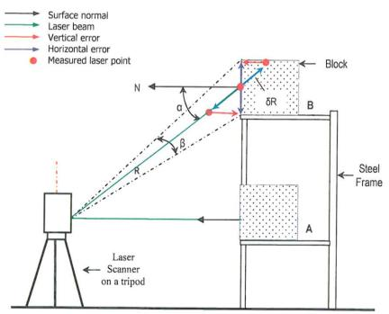
Fig. 1: Scanning the block at normal incidence and the range error at non-normal incidence. Modified from Bitenc *et al.* (2010).
