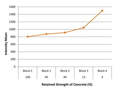
Fig. 7: Intensity vs retained Strength of heated concrete
