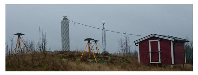
**Figure 2**. The SWEPOS site Vänersborg during a station calibration setup in November 2014. An Eccosorb plate is mounted directly below the choke-ring antenna. Note the typical SWEPOS concrete pillar and the recent steel-grid mast with the LEIAR25.R3 antenna and LEIT radome installed.
