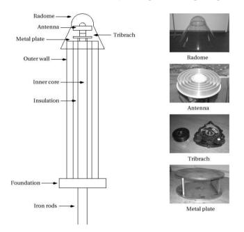
**Figure 1**. Structure of a concrete pillar foundation in SWEPOS, designed in 1992. The pillar height is ~ 3 m, and is anchored onto crystalline rock. Note the relatively large metal plate used as foundation for the tribrach.
