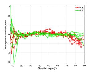
Figure 9. The L1 and L2 residuals when processing the steel-grid mast data with the model with updated general PCV.
