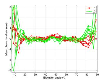
**Figure 8.** The L1 and L2 residuals when processing the pillar data with the model with updated PCV.
