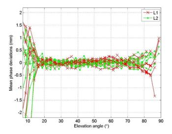
**Figure 4**. Phase deviations of the nine SWEPOS stations investigated when using the updated PCO/PCV description file for SWEPOS antennas. The signature in the region  $15^{\circ}$  to  $75^{\circ}$  is significantly smaller than in Figure 3.
