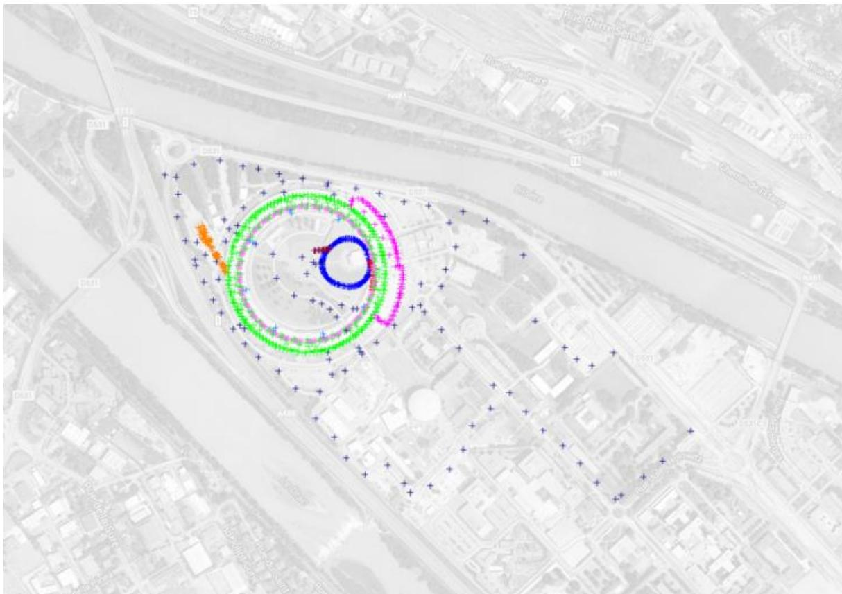
Figure 2 Overview of the different main ESRF survey networks.
