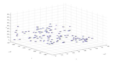
Figure 1. The Samsun triangulation network
