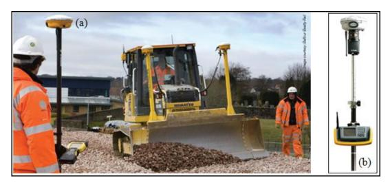
Figure 2: (a) GNSS-Activated Leveling Bulldozers: (b) Trimble Integrated surveying combines robotic total station with RTK GNSS (<u>www.trimble.com</u>)
