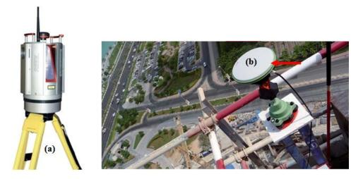
Figure 9: (a) RIEGL VZ-1000 Terrestrial Laser Scanner; (b) Monitoring Vertical Towers with Core Wall Control Survey System (CWCS) (Source: van Cranenbroeck (n.d))
