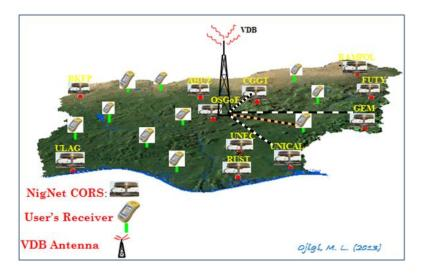
Fig.5: Centralized Network RTK data processing Model for Nigeria (Ojigi, 2014a)
