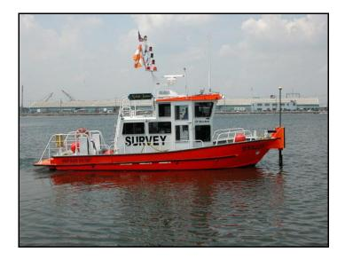
Figure 4: Hydrographic Charting Vessel (<u>http://www.hydrosurveys.net/surveys.htm</u>)
