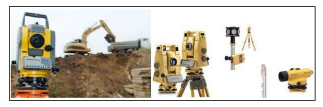
Figure 3a: Electronic Total Station, Theodolite and Laser Levels for Precise Engineering Surveys
