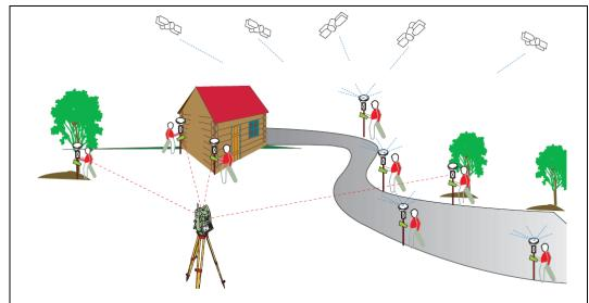
Figure 3b: An Illustration of Surveying with SmartPole (Source: Leica Geosystem (n.d))
