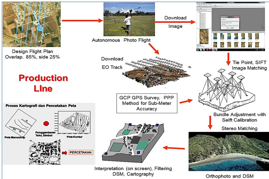
Figure 2. Process Production Utilizing UAV-Based Aerial Mapping
