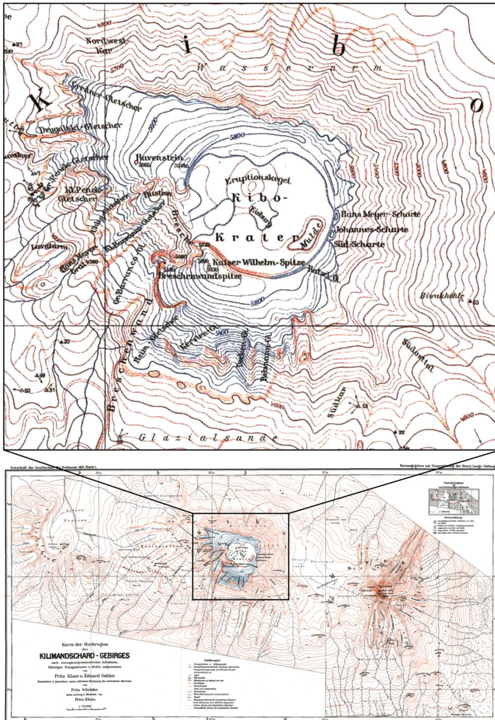
Figure 2. Reproduction of the 1:50,000 scale topographic map of Kilimanjaro derived via ground-based photogrammetry by Klute and Oehler from the 1912 surveying campaign (Klute, 1920).
