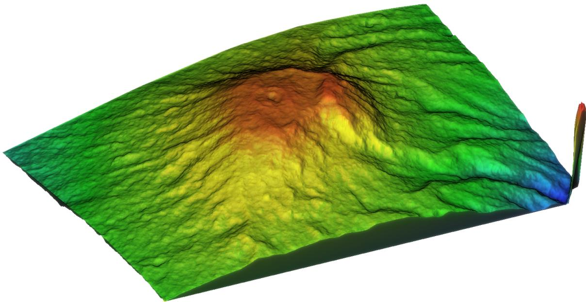
Figure 4. Subset of GDEM V2 on Kibo. Note the “granular” texture of the surface due to the interpolation, as well as the spurious elevation in the Lower Breach Wall area (high peak in the lower right), probably due to clouds in some ASTER stereo pairs.
