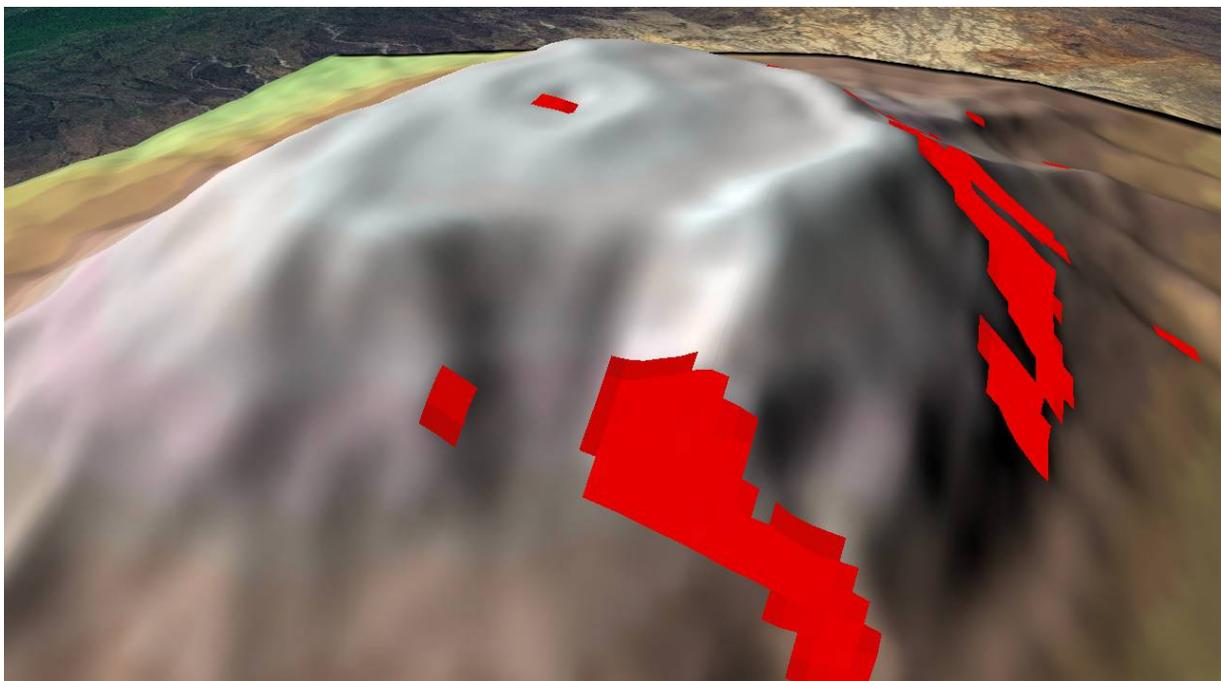
Figure 3. Subset of the Shuttle Radar Topography Mission 90m DEM (SRTM). Data voids are indicated in red.
