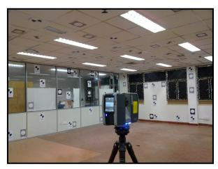
Figure 2: Self-calibration test field for the Faro Focus 3D scanner.
