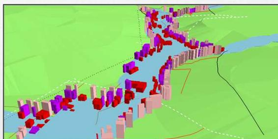
3D Scene of Buildings in ArcScene. The building area extruded based on the buffered distances of 30m (Red), 50m (Purple), and 70m (Brown).
