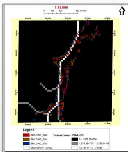
Overlay of buffered buildings (30m,70m,70m) on flow accumulation map to determine vulnerable zones
