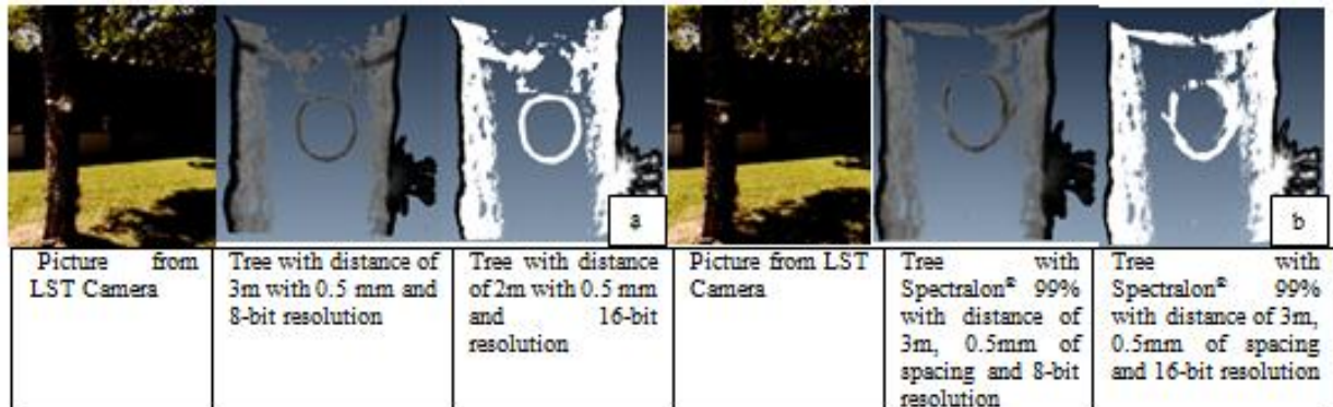
Figure 6. Images produced by the intensity of the LST 3m target with 0.5mm spacing between points and radiometric resolution of 8 and 16 bits.
