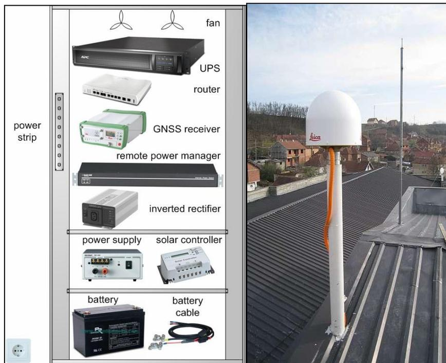
Fig. 5 Equipments placed in the cabinet and the GNSS antenna in one of the stations
