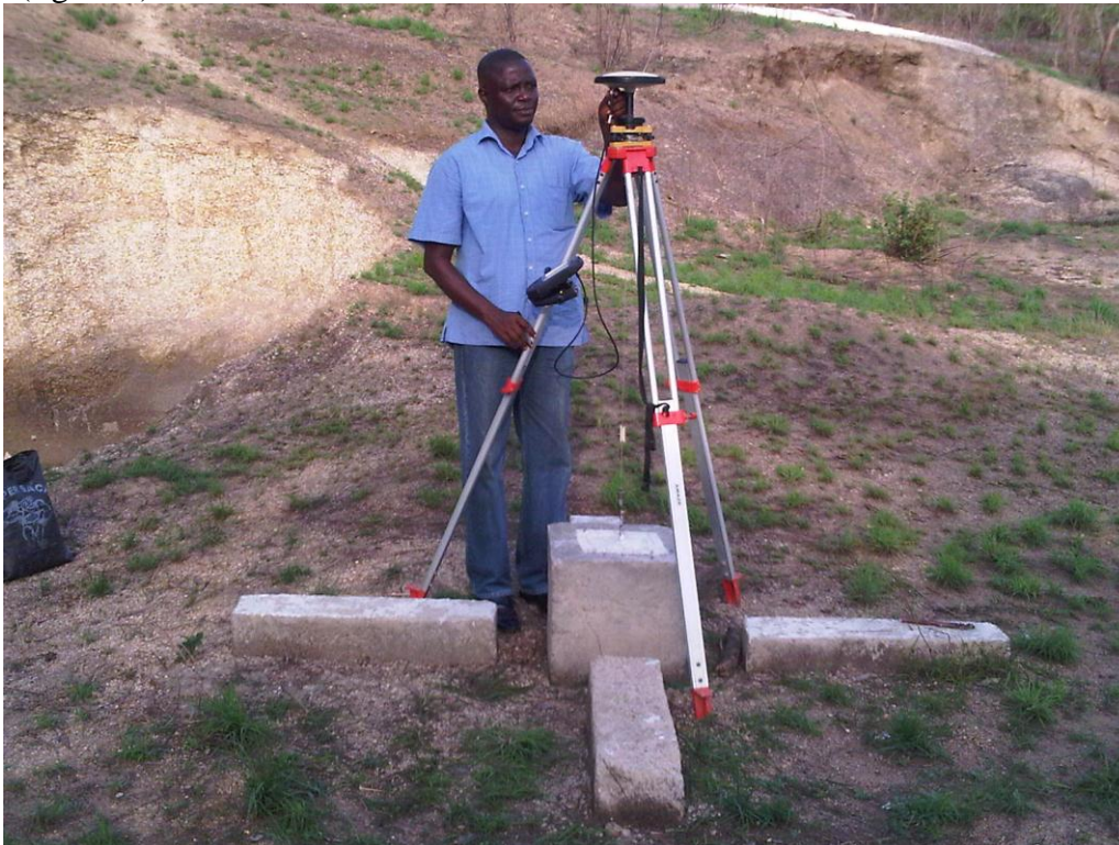
Figure 3: Field Observation with Promark 3
