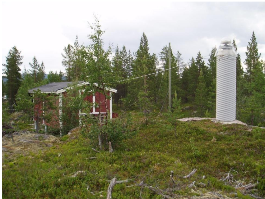
Figure 4: Example of a CORS station (SWEPOS, Sweden)
