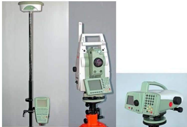
Figure 1: Highly accurate survey instruments: GNSS receiver, total station, level instrument (from left to right), (source: IIGS)
