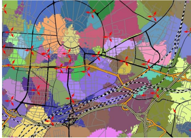
Figure 6: Exemplary mobile phone network with cells and antenna locations and orientations (source: IIGS)
