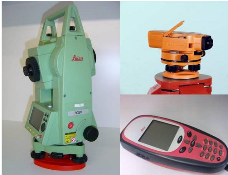
Figure 2: Less accurate survey instruments: total station (left), level instrument (top right), GNSS receiver (downright), (source: IIGS)
