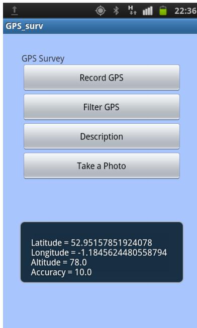
**Figure 3: GPS Survey Application Front Screen**
