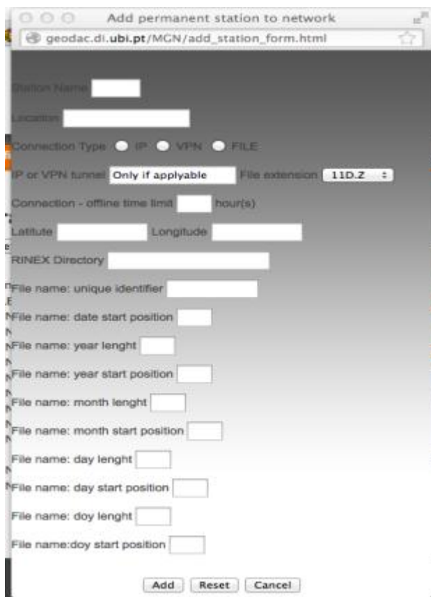
Figure 5 – Example of MGN Pro configuration – Addition of a new station to the network.
