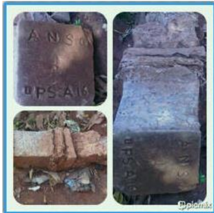
Fig. 3: The Status of GPS A16 (Uprooted)
