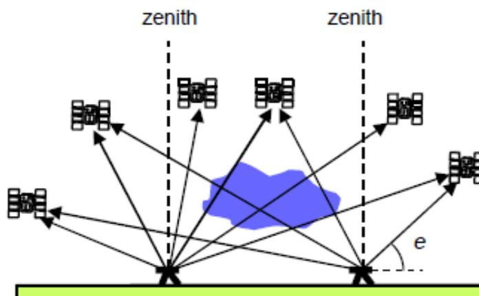
Figure 3 – Zenith Total Delay has a function of the delays for all observed satellites.
