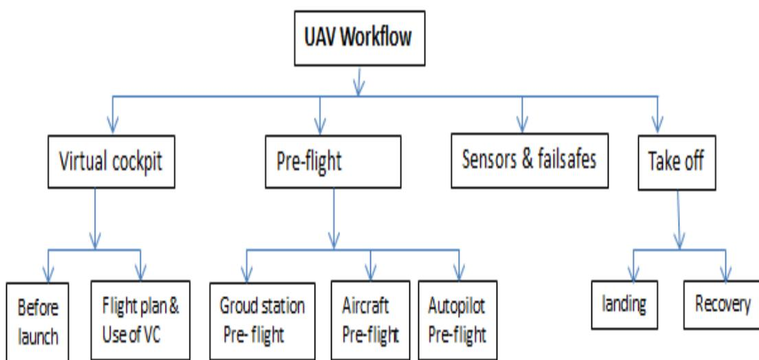
Figure 2 Unmanned Aerial Vehicle workflow.
