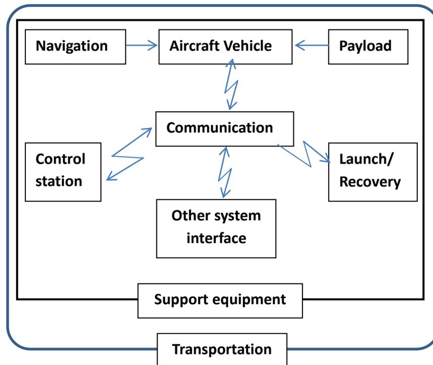
Figure 1 UAV system component
