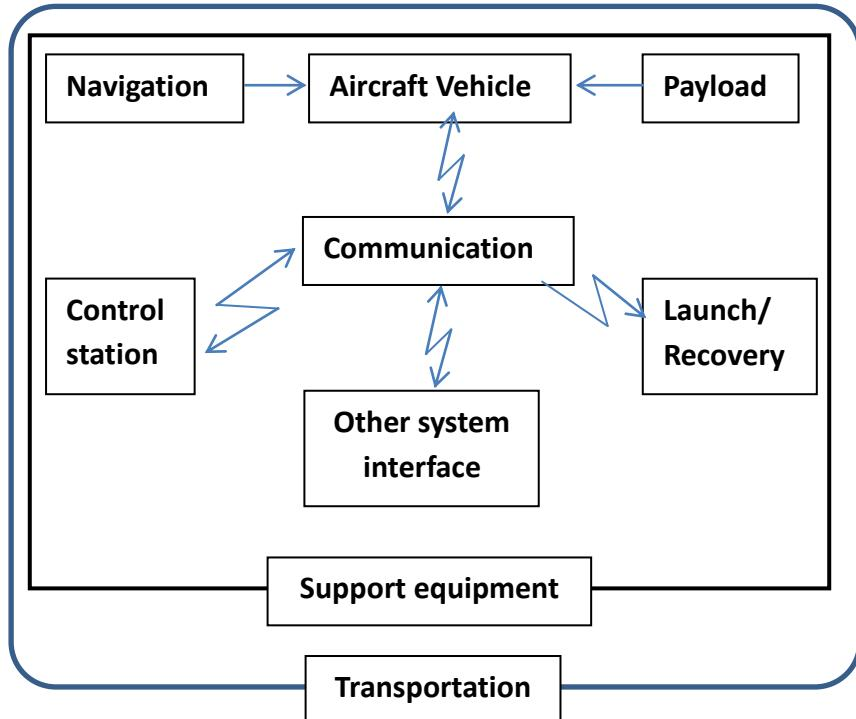
Figure 1 UAV system component
