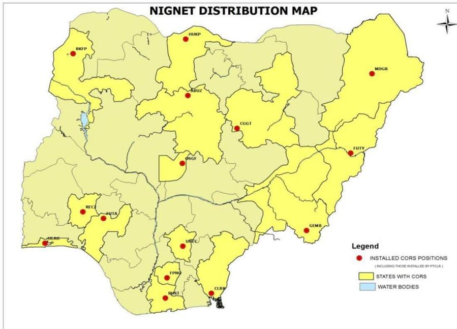
Figure 2: Nigerian Permanent GNSS Reference Network (Edozie and Adebomehin, 2013)
