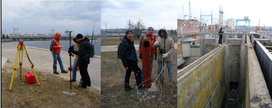
The site survey is an important operation consisting of validating the existing geodesy (coordinate system), the designed location of instrumentation (GNSS and TPS) and to obtain information for the final design validation using "Least Squares Simulation" processing.
