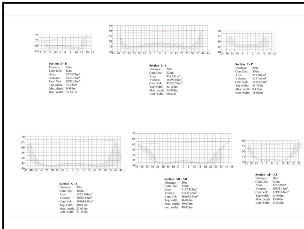
Fig 4: Typical Cross sections of Queen Ede gully
