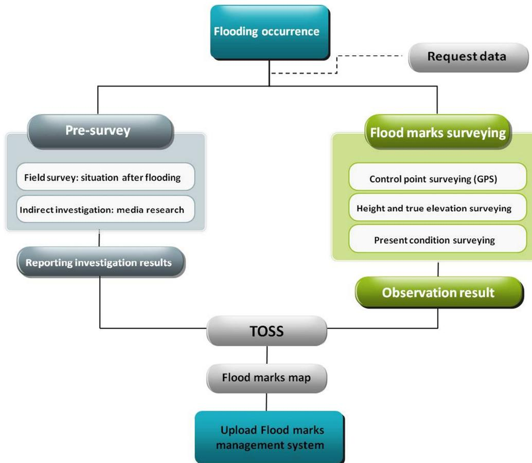
figure 2. Process of making flood marks map
