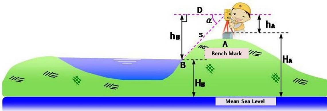
figure 4. Method of true elevation of flood marks
