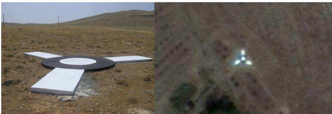
Figure 4.2.4 a) The GCP on the field b) The GCP on the image
