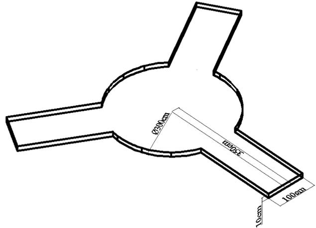
Figure 4.2.1. a ) Steel Frame (from top)
