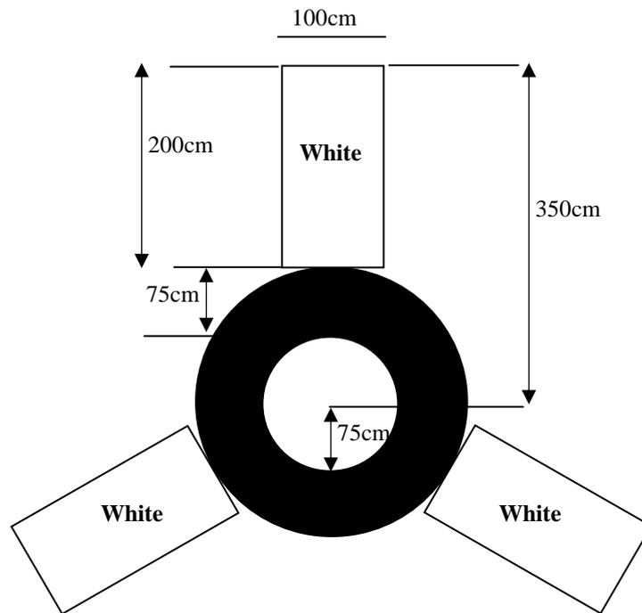
Figure 4.2.3: Dimensions of GCP
