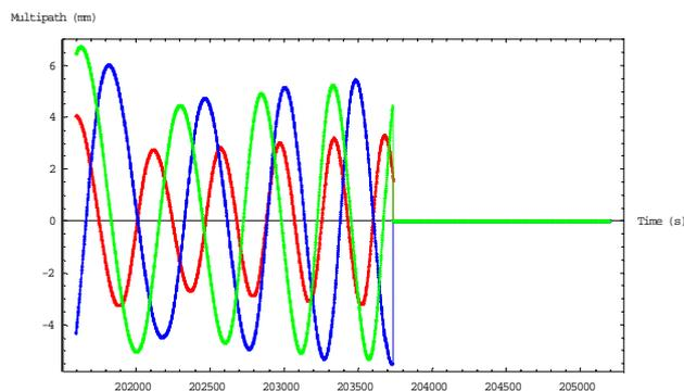
Fig.9. Simulated Galileo three-frequency (red: L1, blue: E5a, green: E5b) multipath error in SV20.
