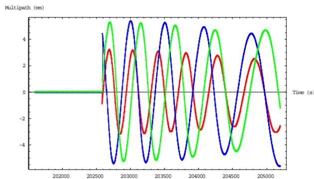
Fig.8. Simulated Galileo three-frequency (red: L1, blue: E5a, green: E5b) multipath error in SV14.
