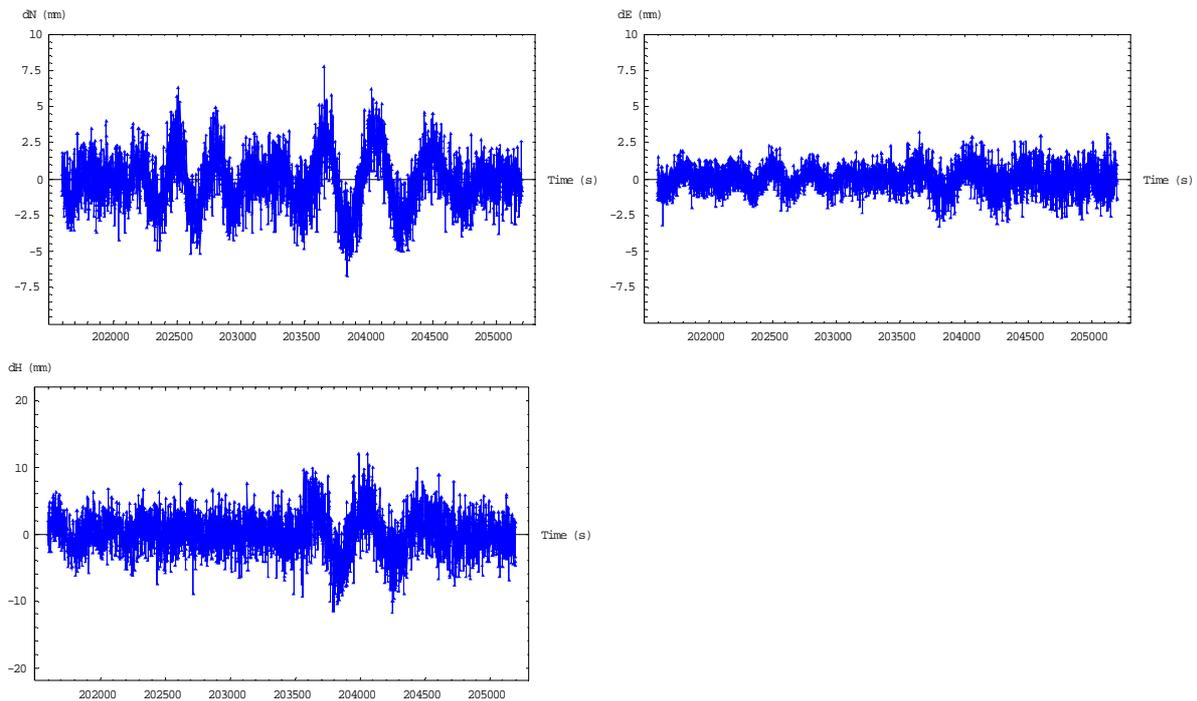
Fig.3. Positioning error in northing (top left), easting (top right), and vertical (bottom left) of single-epoch solution using GPS dual-frequency data.
