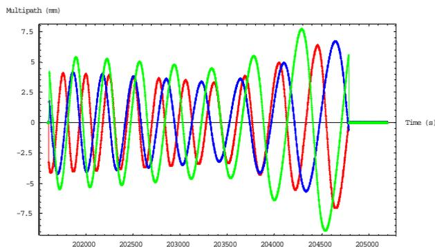
Fig.7. Simulated GPS three-frequency (red: L1, blue: L2, green: L5) multipath error in PRN02.
