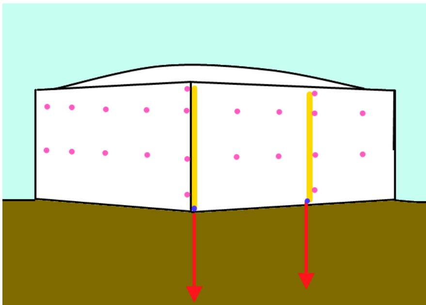
*Fig. 12: View of the building from the total station, reflectors and geotechnical sensors*
