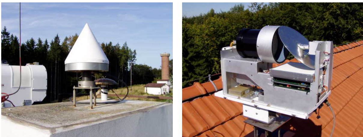
Figure 1: GNSS antenna (left) and Water Vapour Radiometer (right) at GOPE
