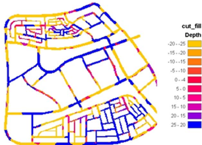
Figure 7. Map of the cut and fill depths for the city road network.
