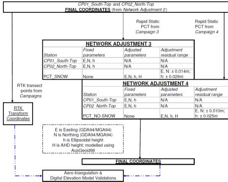
Figure 7: *Network Adjustments 3* and 4, photo control points.
