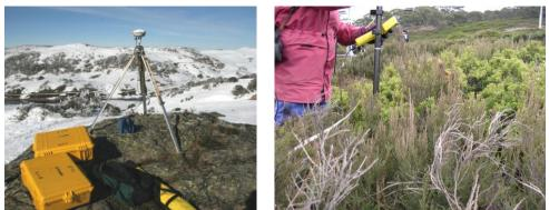
Figure 3: (a) (left) Static GPS setup, *CP01\_South-Top*, during *Campaign 3* and (b) (right) RTK survey in tall shrubs.
