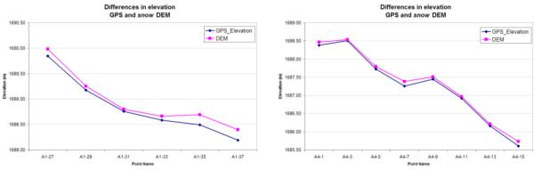
Figure 8: (a) (left) Survey site A1, 60 m transect and approximately 12 m between points and (b) (right) Survey site A4, 70 m transect and approximately 10 m between points.
