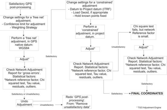
Figure 5: Network adjustment flow-diagram.
