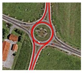
Additional internal data checks are possible. Special road feature like crossings and roundabouts are feasible. Fig. 8 shows an example of a test for a roundabout. In this test for both accuracies location and height – were checked through driving the roundabout two times.
