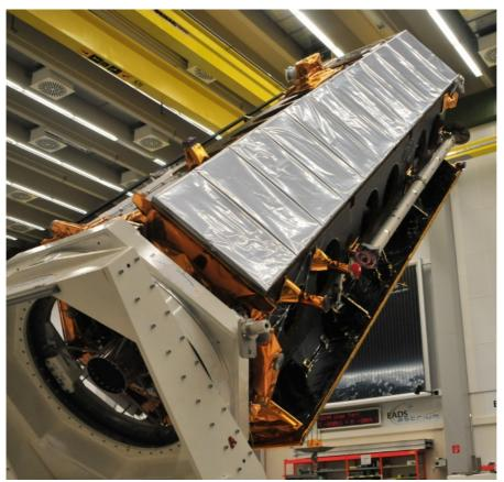
Fig. 2: SAR panel of TanDEM-X satellite
