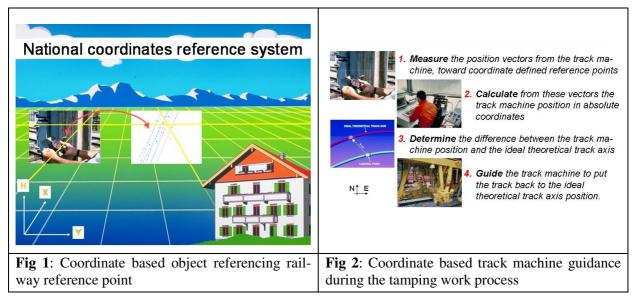
The fully automated 4 steps tamping work process steers the physical operations (Fig 2):
