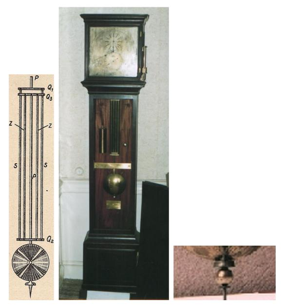
Fig. 4: Crossbar Q2 is suspended from Q1 by two steel bars (S). Crossbar Q2 moves lower when the steel bars (S) expand and lowers the pendulum bob, crossbar Q3 moves higher when the zinc bars (Z) expand and lifts the pendulum bob which is suspended from Q3. The right choice of lengths of the bars with different expansion coefficients creates temperature compensation. After Jordan & Eggert, (1948), Handbuch der Vermessungskunde (left).
