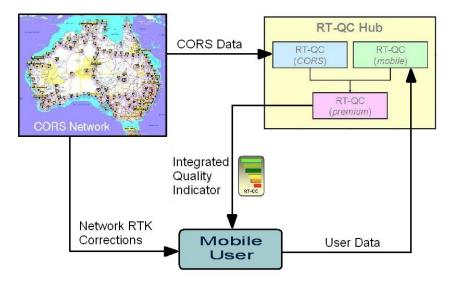
Figure 3. RTQC Mobile Setup
