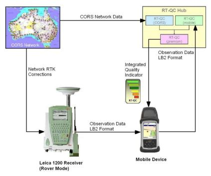
Figure 5. Leica Rover Set Up.
