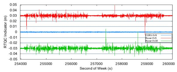
Figure 8. Individual RTQC Indicators during railway survey on 1<sup>st</sup> April 2009.
