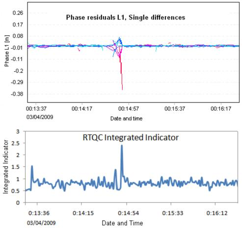
Figure 9. L1 Phase residuals and RTQC Integrated Indicator
