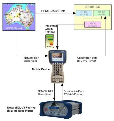
Figure 4. Novatel Moving Base Set Up.
