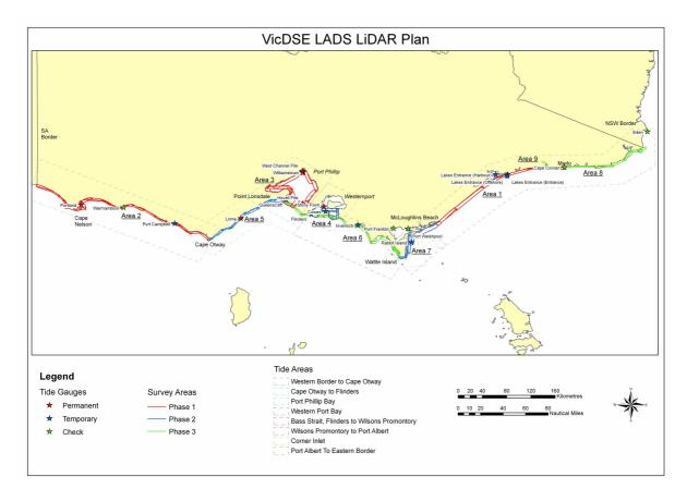
This approach ensured that the surveys were progressed in an order corresponding to the VicDSE priorities. It further ensured alternate areas were available on the west coast, east coast and in a sheltered bay during each phase, in the event of poor environmental conditions. It also followed the important survey maxim of divide and conquer, which enabled areas to be completed progressively, in lieu of trying to survey the entire coast as a single activity.
