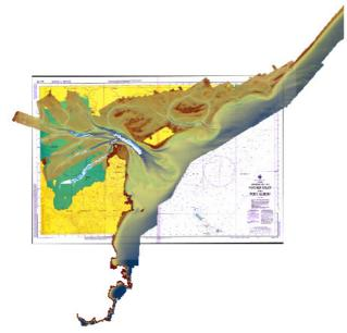
In this image, the offshore data from the coastline to seaward of the 20 m isobath and deeper areas within corner inlet were collected using the LADS Mk II system. The data within Corner Inlet to a depth of approximately 10 m was collected using a combination of LADS MkII and Hawk Eye II systems.
