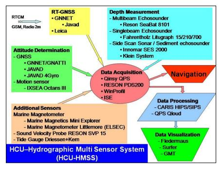
Figure 1: The HCU-Hydrographic Multi Sensor System
