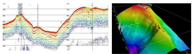
Figure 6: Pockmarks in the Lake Constance. Left: Subbottom profiling of active and inactive pockmarks, Innomar SES 2000. Right: Multi beam echo sounding DTM (from: *Böder and Wessel 2008*)
