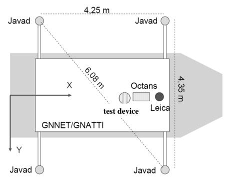
Figure 4: Possible configuration for an investigation of attitude sensors
