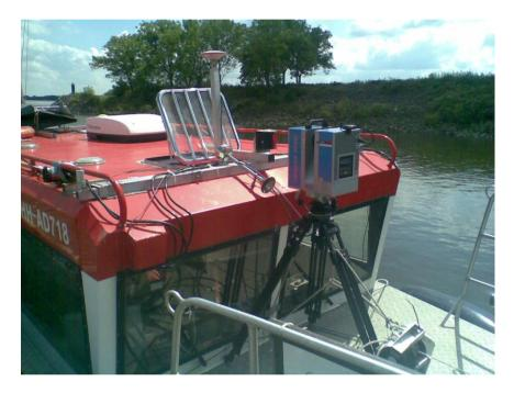
Figure 10: Installation of a terrestrial laserscanner from Zoller&Froehlich (owner: company DHPI) onboard the Level-A
