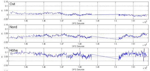
Fig. 3: Difference between RTK and PPP solution in East (Ost), North (Nord) and Height (Höhe) in the balance point of the four antennae.
