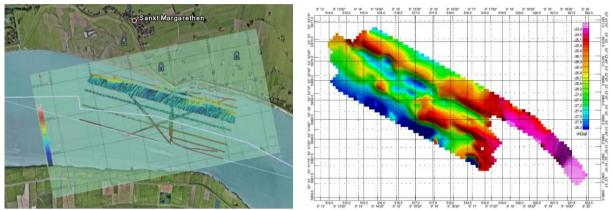
Figure 7: Profiles (left) and free air anomalies (right) measured with the HCU-HMSS and the gravimeter CHEKAN AM from Gravionic.
