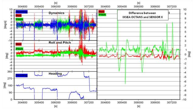
Figure 5: Left: Dynamics in heading, roll and pitch [deg/s]; roll, pitch, heading in [deg]. Right panel: Difference between IXSEA OCTANS III and attitude sensor X in [deg].
