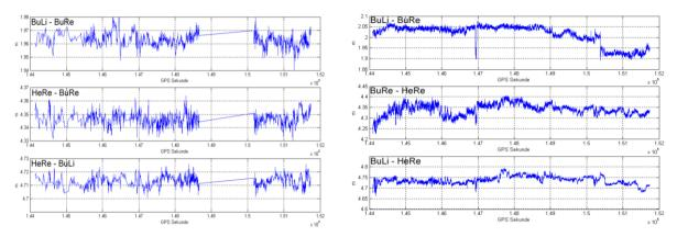
Fig. 2: Distances between GNSS antenna onboard the Level-A. Left: determined with RTK positions, right: determined with PPP positions. Different scales used.
