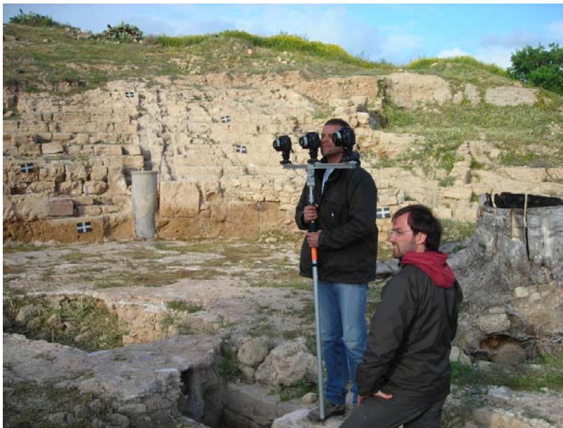
Fig.2 : Close range photogrammetry.
