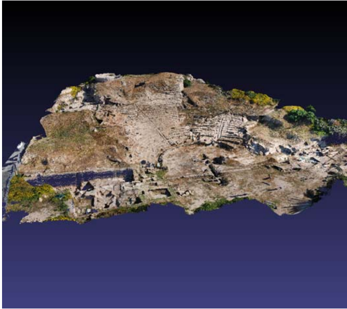
Fig.3: Point cloud of the whole area of the Theater from aerial photogrammetry.
