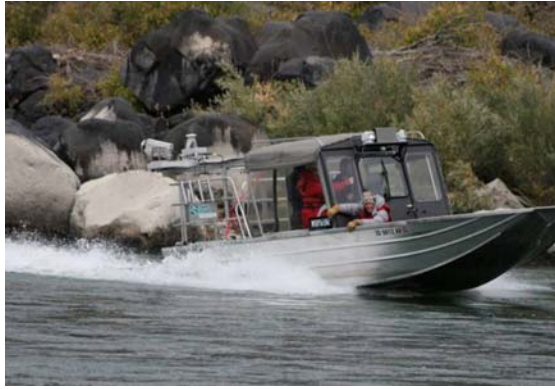
Figure 5. LYNX Mobile Mapper™ installed on a jet boat (left) and an image of data point cloud (right)
