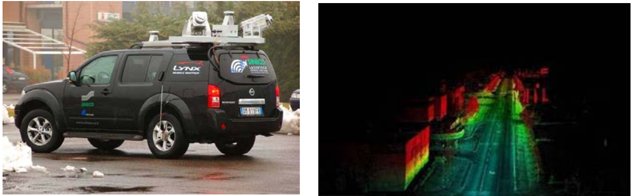
Figure 3. LYNX Mobile Mapper™ installed on a minivan (left) and an image of data point cloud (right)
