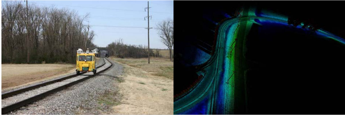
Figure 6. Switchers and turns of a railway road could be easily mapped by LYNX Mobile Mapper™
