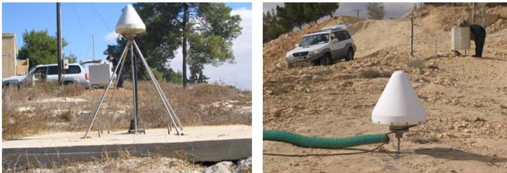
*We would like to examine the effects of the antenna height on pseudorange multipath in a variety of GPS antenna types.*
