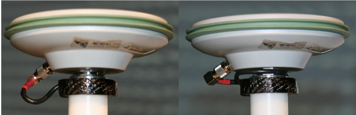
Fig. 7: Differences in cable placement.
