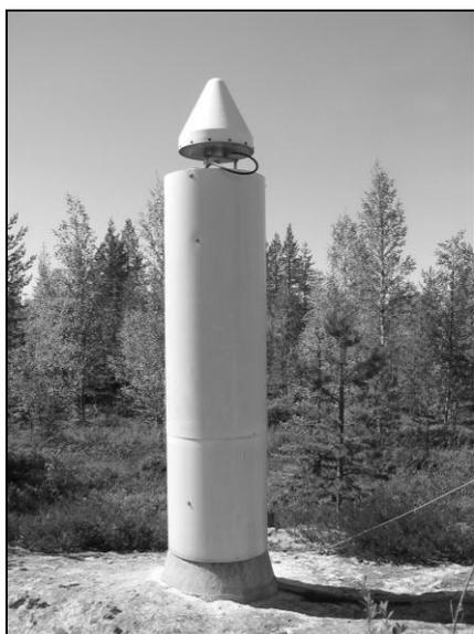
**Figure 2.** A pillar of Romuvaara permanent GPS station. Three FinnRef<sup>®</sup> stations have this kind of concrete pillar as antenna platform. Same kind of pillars is used on the geodynamical test fields used in this study as well.
