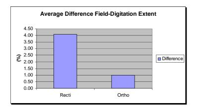
Extent difference of the highest object at rectification is 146.615  $\text{m}^2$  and for the lowest object is 8.117  $\text{m}^2$ . In orthorectification extent difference of the highest object is 19.357  $\text{m}^2$  and the lowest is 1.006  $\text{m}^2$ .
