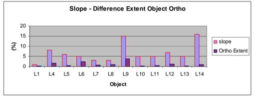
After comparing that, we can see the trend of increasing difference is equal to the increasing slope from the accordance object. And so, the slope difference affect to extent difference that resulted by ortho images digitations.
