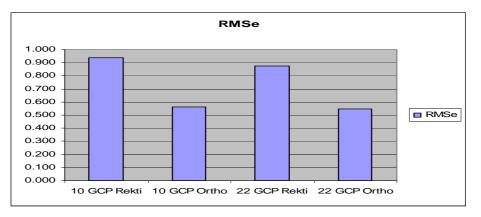
From what can be seen above, images accuracy that is resulted by orthorectification process have a less geometric error, than rectification process without using DEM.
