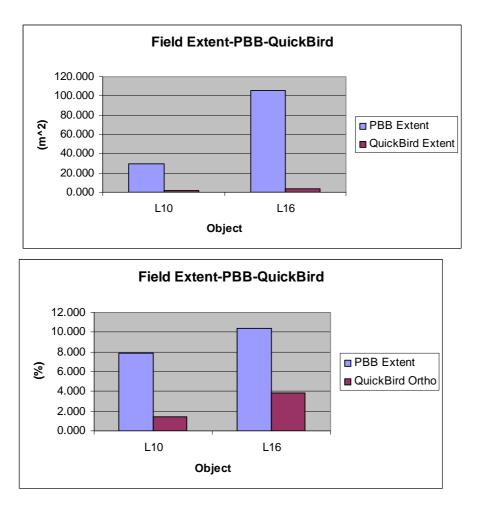
Basic on calculation and graphic at above picture, The percentage of extent difference, the percentage average of extent difference between field extent and PBB spatial data is 9 %. The percentage average of extent difference between field extent and digitation result of orthorectified images is 3 %. There is an escalation of rigorous of tax object extent to be 3 times using orthorectified images on this research.
