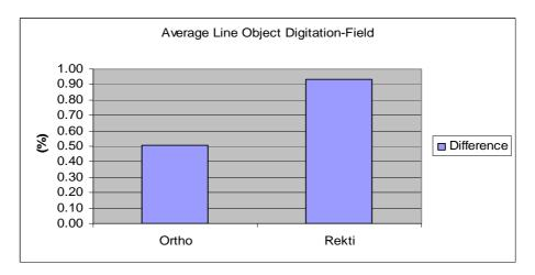
From digitations and field measurements, we can see that the tendency of digitations accuracy of the orthogonal images that already going through the orthorectification process, is better than the one from rectification process.
