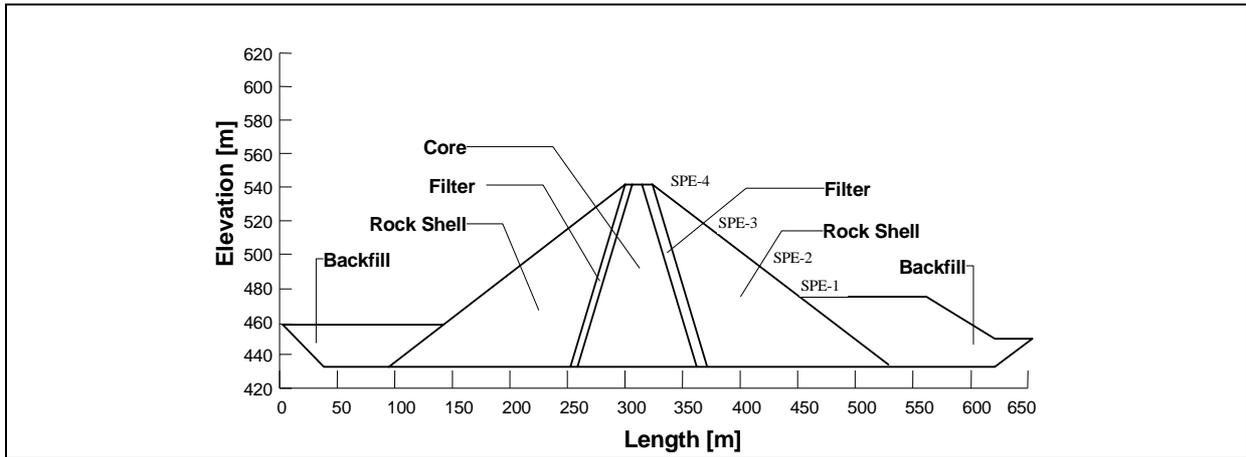
**Figure 1.** Schematic cross-section of the West Dam
