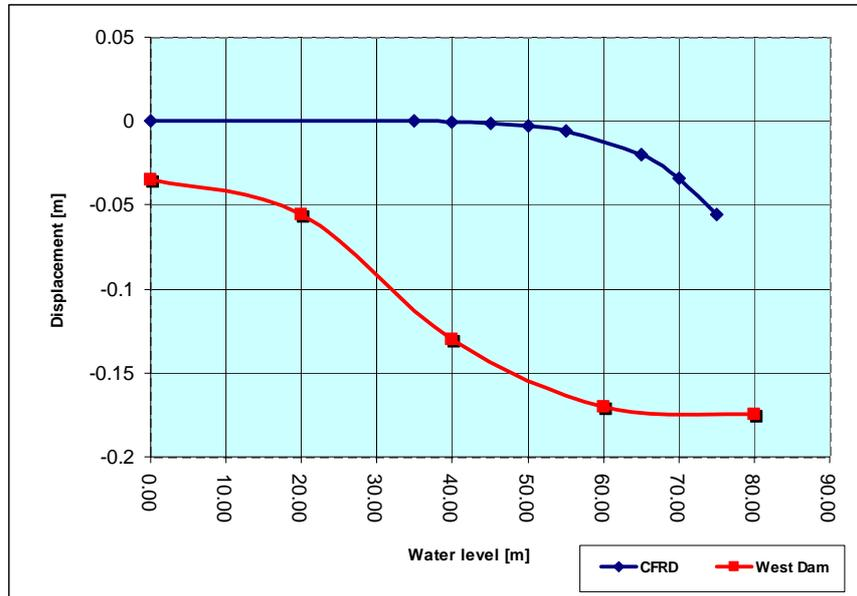
**Figure 4.** Settlement of crest during filling up a reservoir
