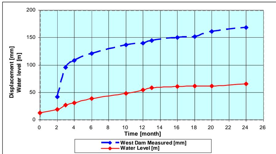
Figure 6. Settlement of the crest of the West Dam during filling up a reservoir as a function of time
